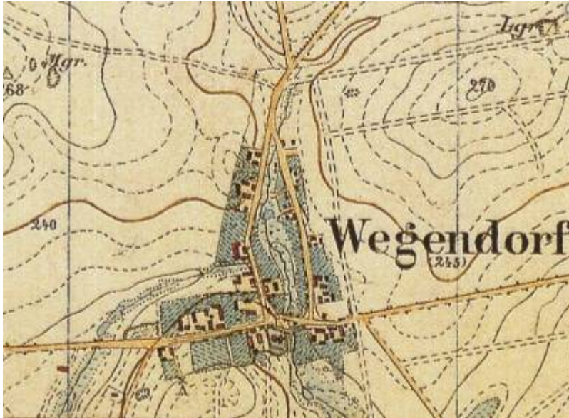
Fig. 13: Indicating elevation contours on a
