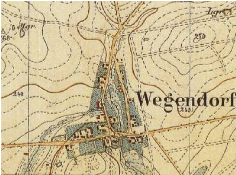
Fig. 13: Indicating elevation contours on a map
