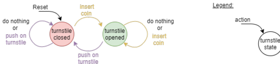
Fig. 12: State Transition Diagramm of the Entrance Control for Toilets
